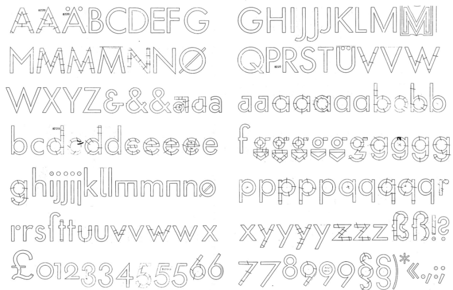
Figure 23. Character outlines incised in copper plates used as patterns for engraving the matrices of 20-point regular weight Futura. Extracted from Bauer foundry intaglio proofs, as reproduced in Burke, Paul Renner: The Art of Typography , 92–93.
